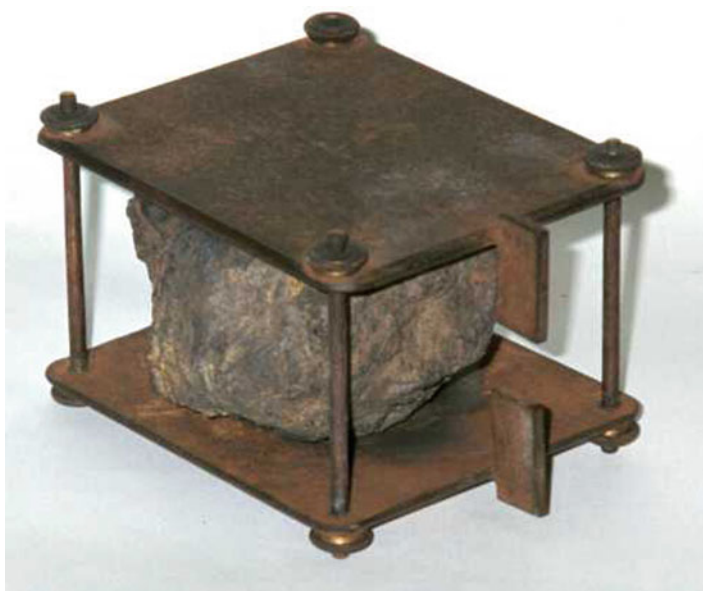
Fig. 4.2 A lodestone sandwiched, as if it might inexplicably fly away, between two iron plates. A strong magnetic field is established between the two vertical vanes (Image courtesy of Westminster College, Pennsylvania: http://physics.kenyon.edu/EarlyApparatus/index.html )
